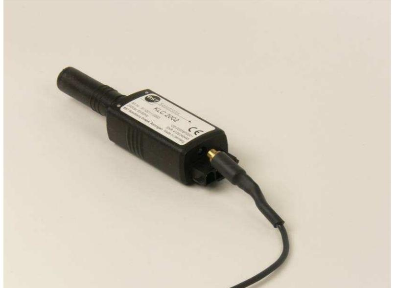
The moment the device is connected and supplied with power the data link starts and the LED on the interface starts to blink.
